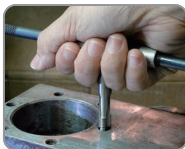
2. Tap re-drilled hole using tap
