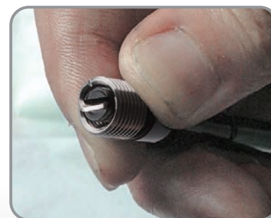
3. Load coiled insert into applicator
