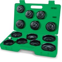
TOPTUL cup-type oil filter wrenches are made of gauge construction and are able to withstand up to 85 ft-lbs of torque applied. The cup-design grip functions as a socket minimizing the possibility of crushing filters and fits both 3/8" and 1/2" (adapter) square drive tool. The cups are coated with electro-black oxide finish for long life protection against rust
