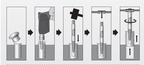
To use, a small hole needs to be drilled in the centre of the rogue screw and the correct sized extractor inserted. The extractors are threaded in the opposite direction to conventional screw threads. When the extractor is tightened in an anti-clockwise direction, it begins to loosen the screw.
