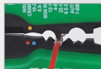
Non-insulated terminal crimping
