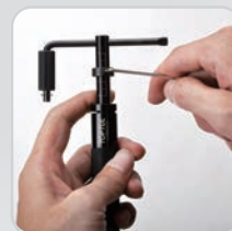
2. Set-up locking block to adjust coil insert depth
