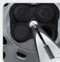
5. Using Pliers, take off pin on insert
