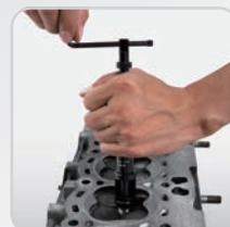
4. Screw coil into thread slowly
